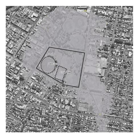
As the land is flood prone all structures will require a risk analysis report to demonstrate they are structurally adequate along will ensuring that all materials below the 1% AEP level are flood compatible.
